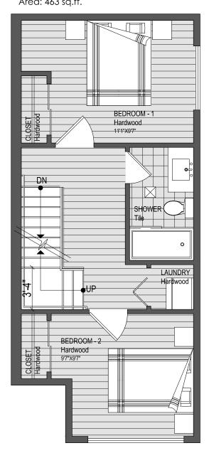
1st FLOOR PLAN(LOCK-OFF UNIT)
